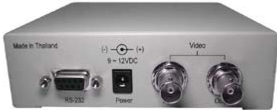
Figure 11: TDCT-Pro Rear Panel and Connections
