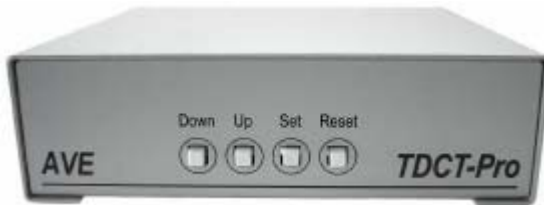
Figure 1: Four Front Panel Push Buttons of TDCT-Pro
